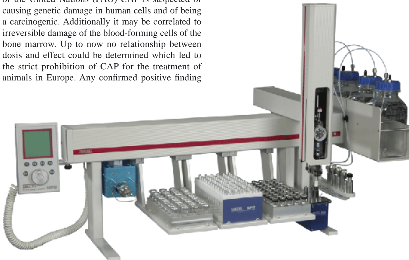
Figure 2. GERSTEL MPS with integrated SPE option, solvent reservoir and injection valve.
