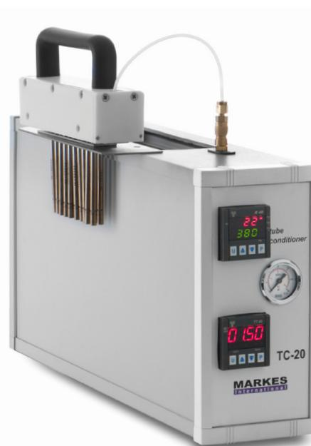
The TC-20 uses a flow of clean nitrogen to condition or dry-purge up to 20 industry-standard stainless steel, inert-coated or glass sorbent tubes at temperatures up to 400°C.
