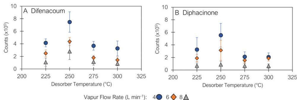
FIG. 1—Optimization of the thermal desorber temperature (x-axis) and Vapor flow rate (different series) for difenacoum (A) and diphacinone (B). Integrated peak areas of the protonated molecule from the extracted ion chromatographs (EICs) are plotted. Error bars represent the standard deviation of 5 replicate measurements.
