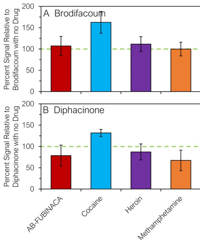
FIG. 5—Response of brodifacoum (A) and diphacinone (B) at a 1:100 rodenticide : drug ratio in negative ionization mode. Error bars represent the standard deviation of three to five measurements.
