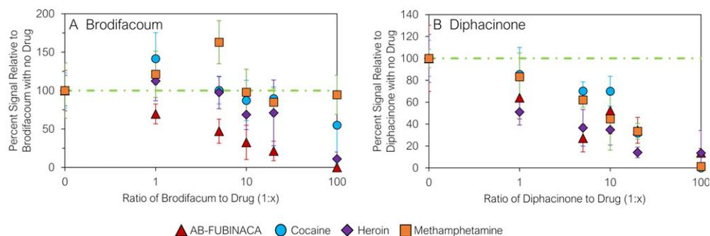
FIG. 3—Competitive ionization studies of rodenticide/drug mixtures. The response for brodifacoum (A) and diphacinone (B) in the presence of increasing levels of AB-FUBINACA (red triangle), cocaine (blue circle), heroin (purple diamond), and methamphetamine (orange square). The green dotted line represents the level of the rodenticide with no drug present. Note that the x-axis is plotted on a log scale.
