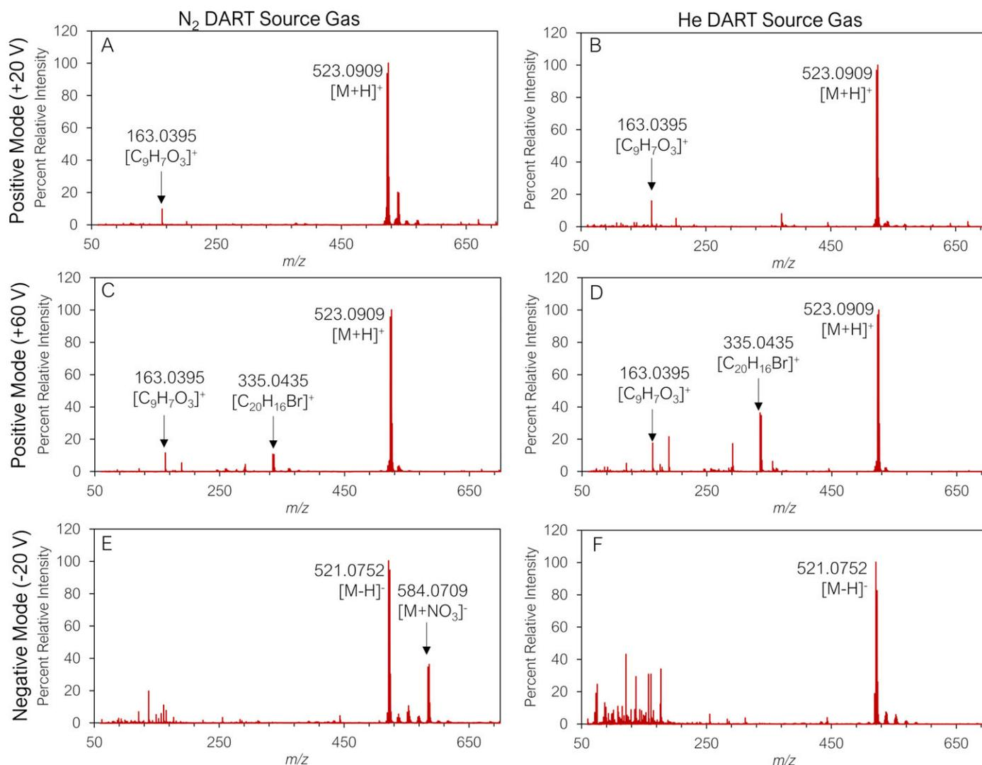
FIG. 2—Representative mass spectra of brodifacoum using nitrogen (A, C, and E) and helium (B, D, and F) as the DART ionization gas in positive mode (A through D) and negative mode (E and F). For positive mode, both a low fragmentation orifice 1 voltage (A and B) and a higher fragmentation orifice 1 voltage (C and D) are shown. For negative mode, only the low fragmentation orifice 1 spectra (E and F) are shown. Additional representative mass spectra can be found in Figures S1–S7.
