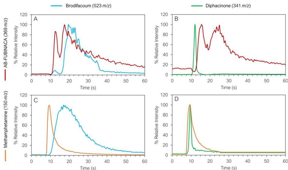
FIG. 4—Extracted ion chromatograms (EICs) of rodenticide drug mixtures. Mixtures of brodifacoum (blue) and AB-FUBINACA (red) (A), diphacinone (green) and AB-FUBINACA (red) (B), brodifacoum (blue) and methamphetamine (orange) (C), and diphacinone (green) and methamphetamine (orange) (D) are presented.
