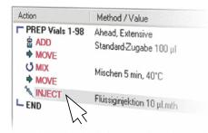
MAESTRO Software enables Sample Prep by Mouse-Click. All sample preparation steps are conveniently and easily selected from a drop down menu and added to the method. Example:
