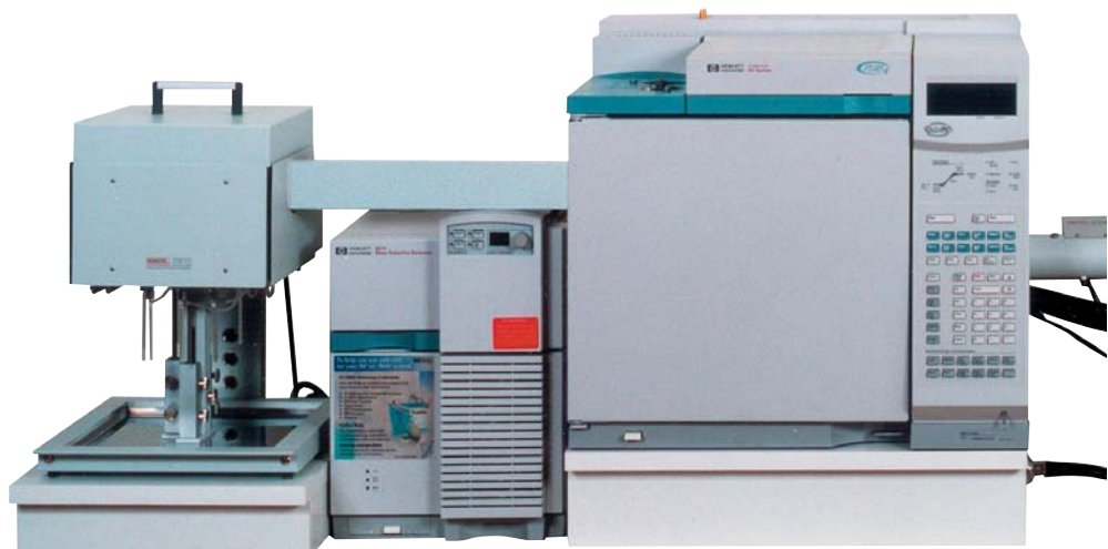
Integrated PFC and Dual Oven DCS-GC/MSD system
