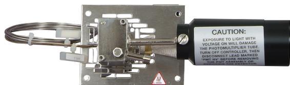
The PFPD is widely used in laboratory and process gas chromatographs to analyze sulfur species and total sulfur levels in liquid-phase petrochemicals.
